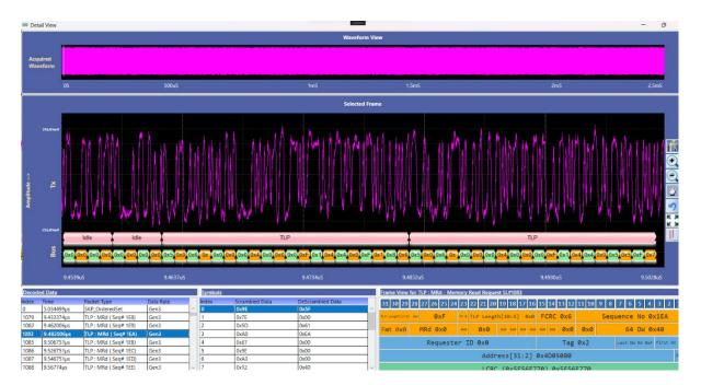
This solution helps in debugging the protocol layer issues and correlating it to physical layer resulting in a reduction in debugging time.
