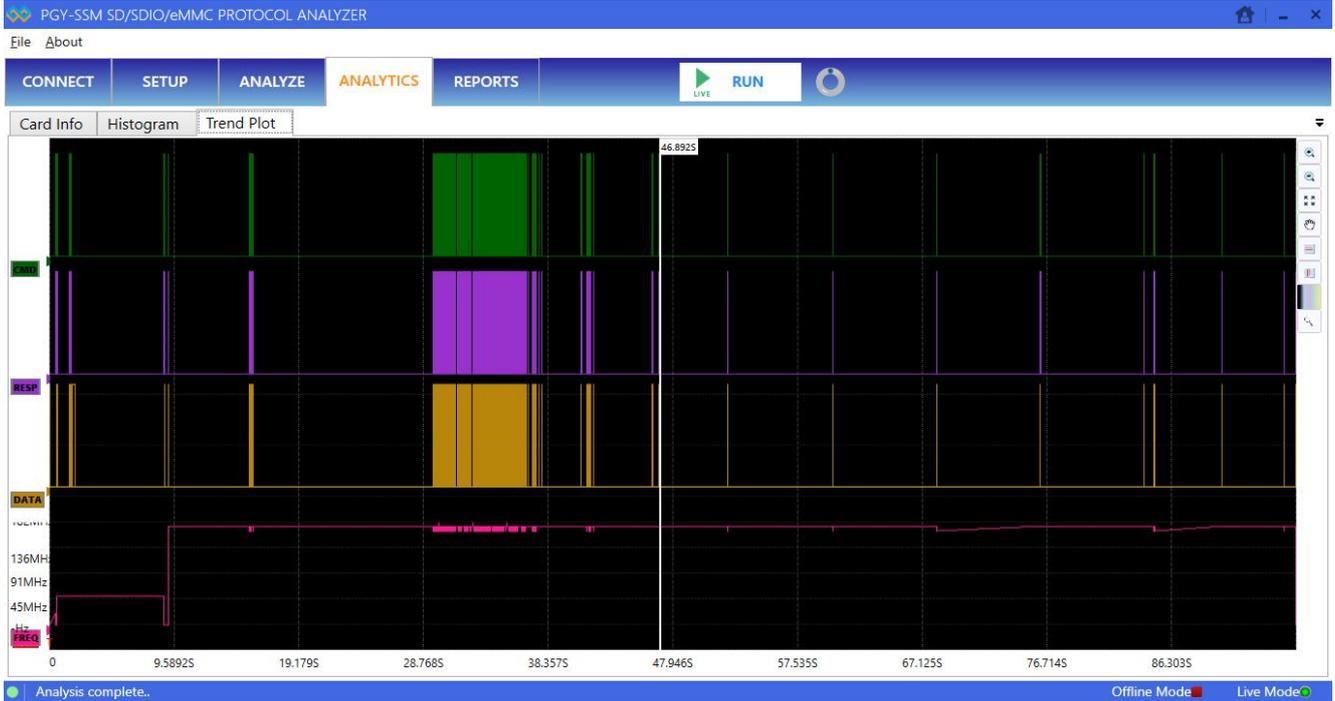
The Analytics view is a bird's eye view of protocol activity for the captured long-duration data. It reduces analysis time by viewing plot command, response, data, and frequency of operation of captured data. The user can search for specific commands or responses in the plot.
