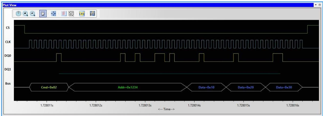
The timing view provides the plot of CS, CLK, DQ0, and DQ1 signals with a bus diagram. Overlaying of Protocol bits on the digital timing waveform will help easy debugging of Protocol decoded data. Cursor and Zoom features will make it convenient to analyze Protocol in the timing diagram for any timing errors.
