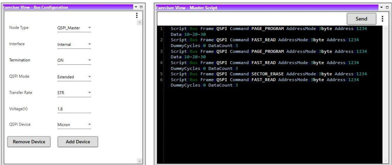
PGY-QSPI-EX-PD supports QSPI traffic generation using GUI and Script. Users can generate simple traffic generation using the GUI to test the DUT. Script-based GUI provides flexibility to emulate the complete expected traffic in the real-world including error injections. In this sample script user can generate QSPI traffic as below:
