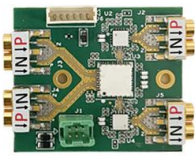
P4012-CTLE-mSMP (UFS4.0 Compatible mSMP Probe tips with CTLE)
