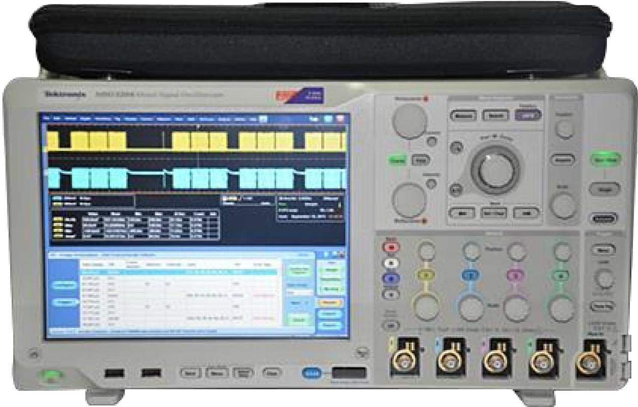
PGY-I3C Software installed in Tektronix oscilloscopes can be launched by clicking on PGY-I3C icon in oscilloscope desktop folder. Now user has simultaneous view and control to oscilloscope as well as PGY-I3C Software. User can analyze I3C in single acquisition mode, Repetitive mode and as well as No Acq mode. In No Acq Mode, I3C software analyses already captured I3C signal that is present in the acquisition memory of the oscilloscope.
