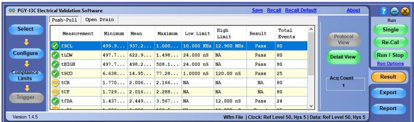
PGY-I3C runs inside the Tektronix oscilloscopes and makes the electrical measurements, and displays the decoded data in a bus diagram, a table, and links the decoded data to electrical signal in the bus diagram.
