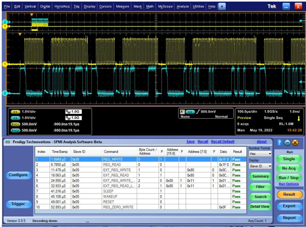
SPMI Electrical Validation and Protocol Decode Software offers electrical measurements compliance testing as specified in SPMI specification. PGY-SPMI Electrical validation and Protocol Decode software runs in Tektronix Oscilloscope provides electrical measurements and protocol decoding at click of button.
