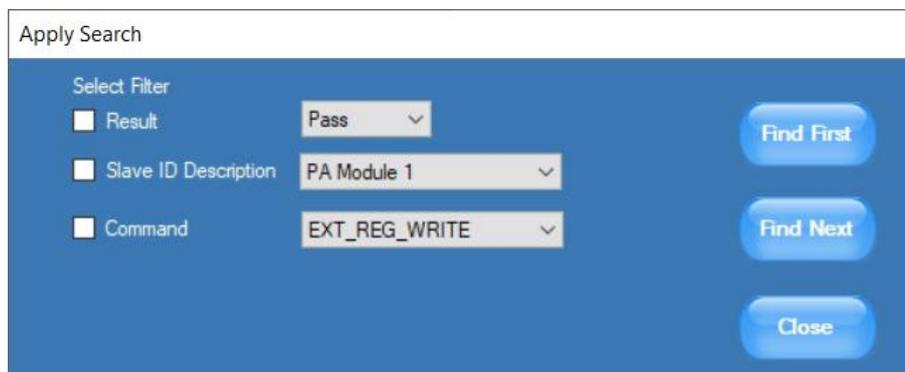
During protocol analysis, users tend to capture a large amount data capture any non-repeatable event. It is also extremely difficult locate the SPMI packet of interest. SPMI Software's Search filter in is able to quickly locate the required Slave ID or command or Combination of both.
