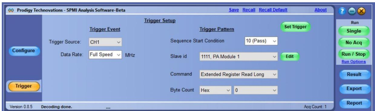
Select any of the live channels Ch1 to CH4 as trigger source and set the trigger pattern. The trigger can set to full speed, half speed or any custom data rate. SPMI provides the flexibility to select a combination of any one of the sixteen slave IDs, any command and command dependent parameters such as Byte count, Address, or Data.
