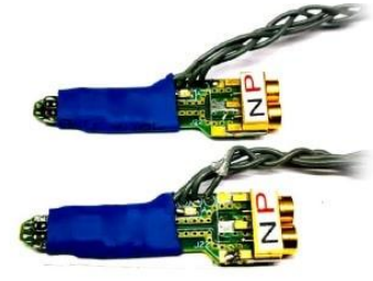
P5021 14 Gbps probe tips for direct access to test points
