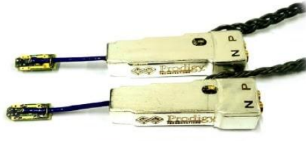
P5021-L 14 Gbps probe tip with isolation resistor
