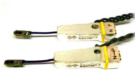
P5021-L-WE 14 Gbps probe tips with passive equalizer at input
