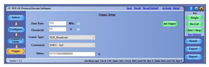
Simple easy to use I3C protocol aware trigger features allows engineers to capture I3C signals at specific event in I3C interface.
