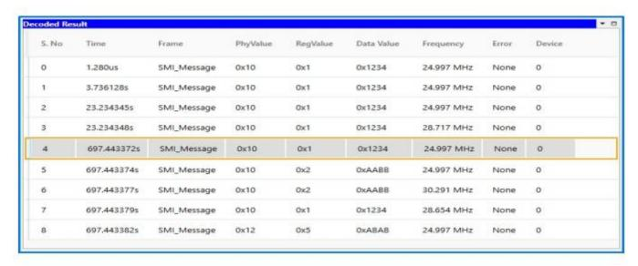
The Protocol window provides the decoded packet information in each state and all packet details with error info in the packet. The Selected frame in Protocol listing window will be auto correlated in timing view to view the timing information of the packet.
