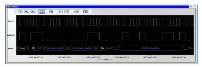
The Timing view provides the plot of MDC and MDIO signals with bus diagram. Overlaying of Protocol bits on the digital timing waveform will help easy debugging of Protocol decoded data. Cursor and Zoom features will make it convenient to analyze Protocol in the timing diagram for any timing errors.
