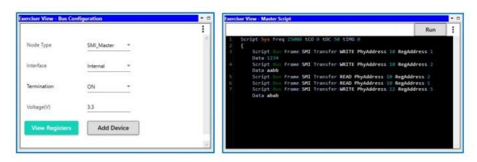
PGY-MDIO-EX-PD supports MDIO traffic generation using GUI and Script. Users can generate simple traffic generation using the GUI to test the DUT. Script based GUI provides flexibility to emulate the complete expected traffic in real world including error injections. In this sample script user can generate MDIO traffic as below:
