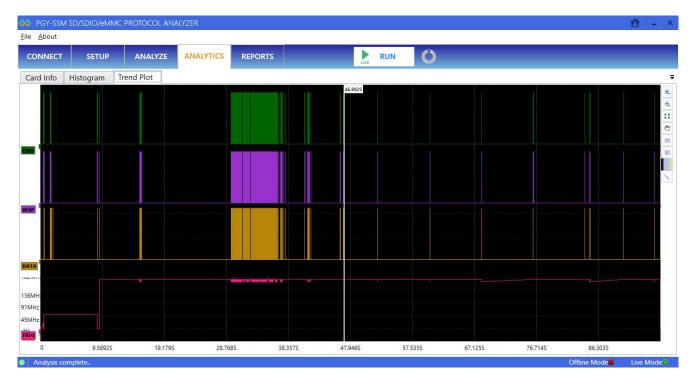
The Analytics view is a bird's eye view of protocol activity for the captured long-duration data. It reduces analysis time by viewing plot command, response, data, and frequency of operation of captured data. The user can search for specific commands or responses in the plot.
