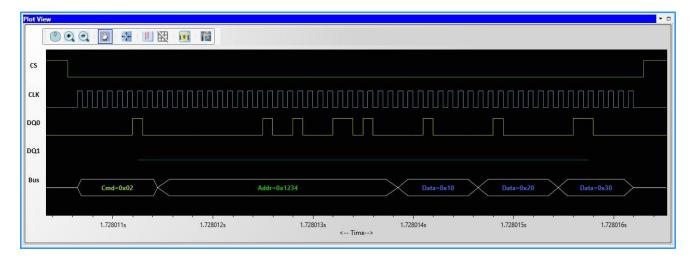
The timing view provides the plot of CS, CLK, DQO, and DQ1 signals with a bus diagram. Overlaying of Protocol bits on the digital timing waveform will help easy debugging of Protocol decoded data. Cursor and Zoom features will make it convenient to analyze Protocol in the timing diagram for any timing errors.
