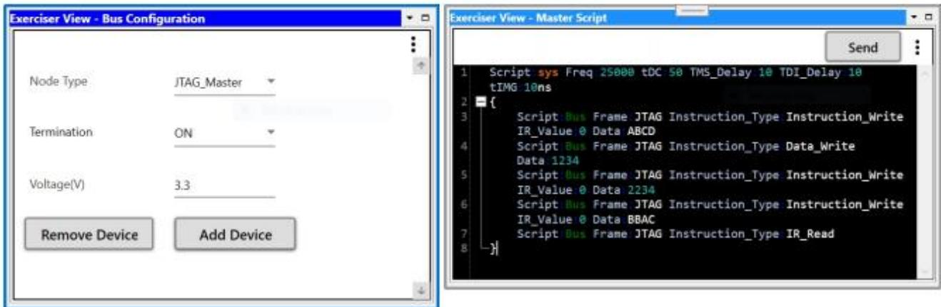
PGY-JTAG-EX-PD supports JTAG traffic generation using GUI and Script. Users can generate simple traffic generation using the GUI to test the DUT. Script based GUI provides flexibility to emulate the complete expected traffic in real world including error injections. In this sample script user can generate JTAG traffic as below:
