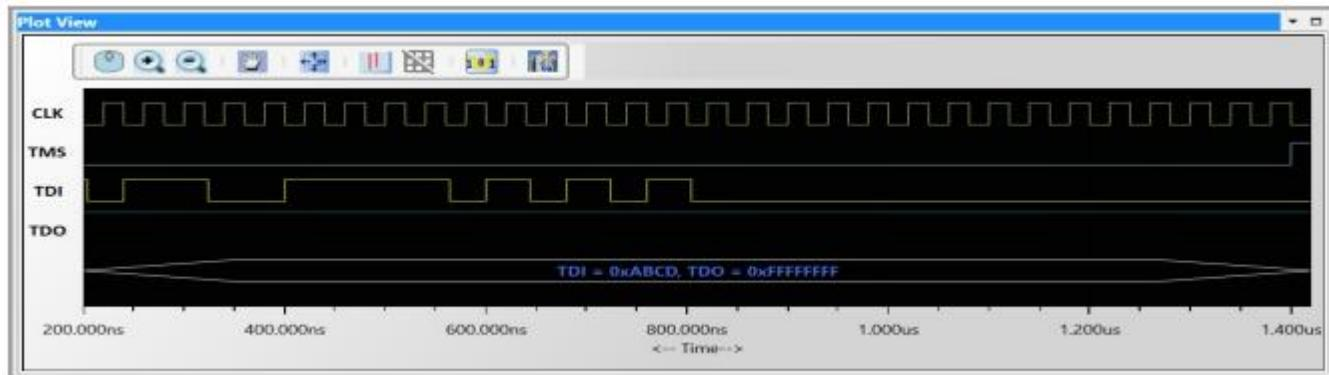
The Timing view provides the plot of CLK, TMS, TDI and TDO signals with a bus diagram. Overlaying of Protocol bits on the digital timing waveform will help easy debugging of Protocol decoded data. Cursor and Zoom features will make it convenient to analyze Protocol in the timing diagram for any timing errors.
