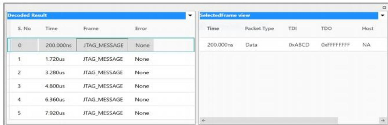
The Protocol window provides the decoded packet information in each state and all packet details with error info in the packet. The Selected frame in Protocol listing window will be auto correlated in the timing view to view the timing information of the packet.
