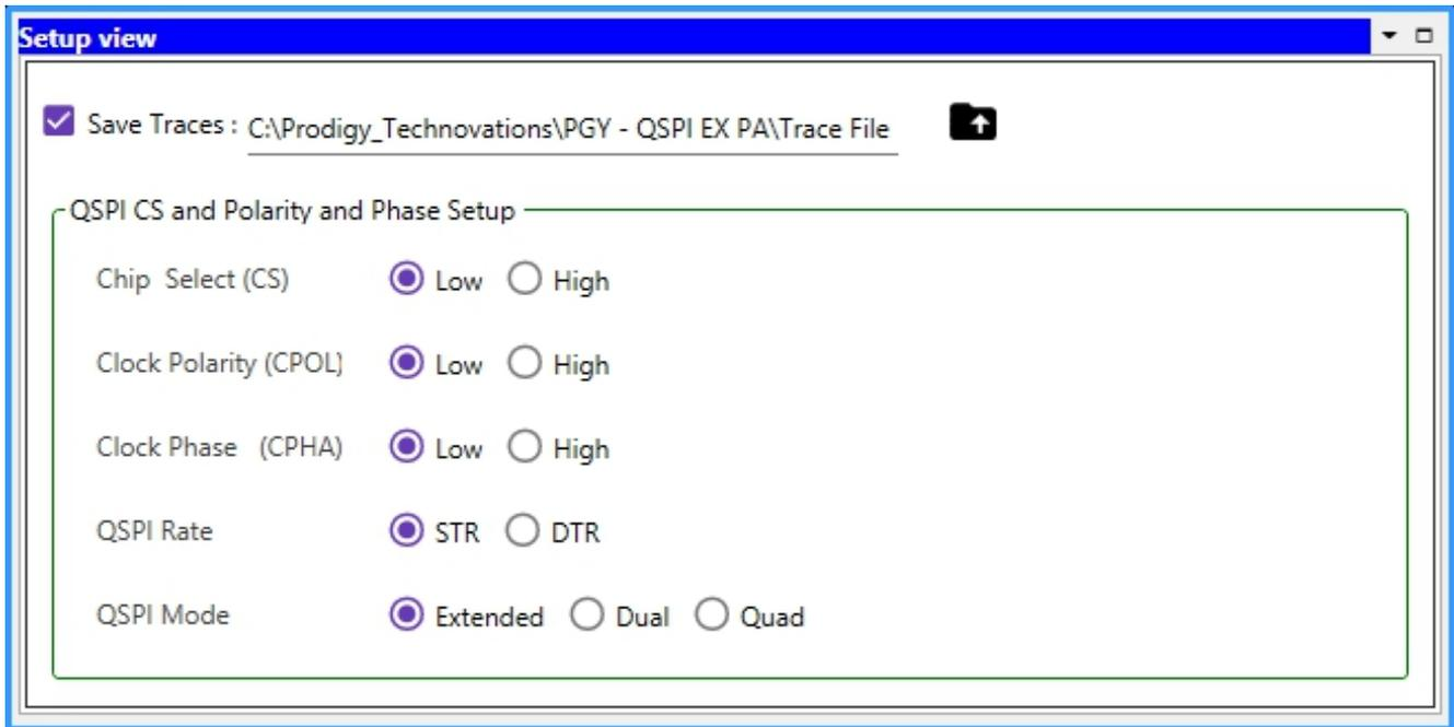
Setup View of PGY-QSPI-EX-PD allows the user to configure the QSPI Chip select (CS), Clock Polarity (CPOL), Clock Phase (CHPA), QSPI rate of STR or DTR and the different modes of QSPI such as Extended, Dual or Quad.
