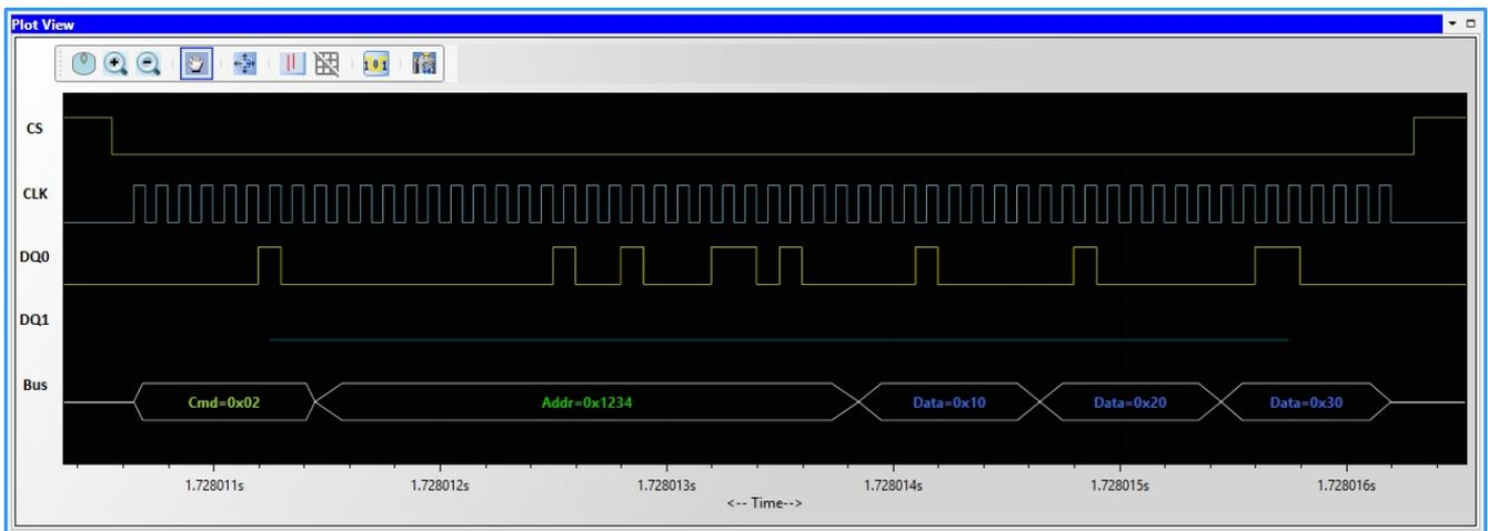
Timing view provides the plot of CS, CLK, DQ0 and DQ1 signals with bus diagram. Overlaying of Protocol bits on the digital timing waveform will help easy debugging of Protocol decoded data. Cursor and Zoom features will make it convenient to analyze Protocol in timing diagram for any timing errors.
