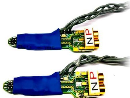
Prodigy Technovations provides innovative solder down active probe tips, which can equalize the MPHY signals upto MPHY HSG5B speed and amplify the signal to support cable loss in mSMP cable and PCB trace in analyzer. These probe tips are tested with real world UFS4.0 host/device test and development platform.
