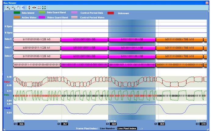
Figure 5: MHL Bus viewer with Physical layer waveforms
