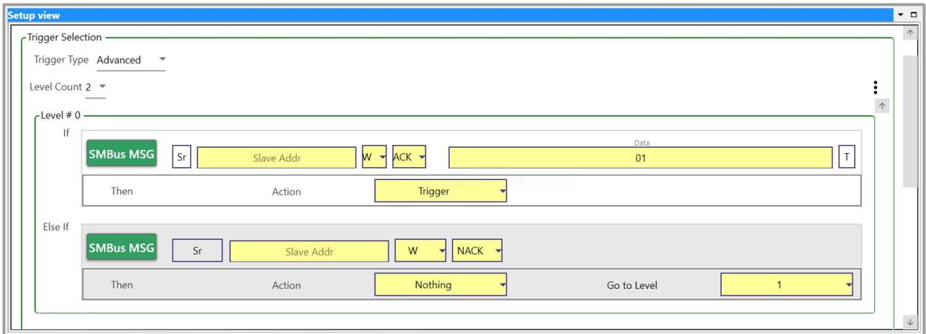
PGY-SMBus-EX-PD supports Auto, simple and advanced trigger capabilities. Analyzer can trigger on any of the SMBus Protocol packets. Advanced Trigger provides the flexibility to monitor Multiple trigger conditions and can set multiple state trigger machine.
