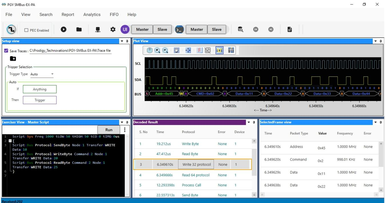
The screenshot displays the PGY SMBus-EX-PA software interface. The top menu includes File, View, Search, Report, Analytics, FIFO, and Help. The toolbar contains various icons for file operations and analysis. The main window is divided into several panels:
