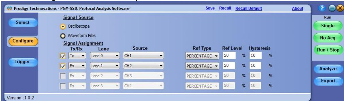
PGY-SSIC MIPI-SSIC Protocol Analysis Software runs inside the Tektronix high performance windows oscilloscopes. Engineers can configure PGY-SSIC Software to automatically import the data from oscilloscopes live channels or wfm file format. This enables live and offline protocol testing of SSIC protocol.
