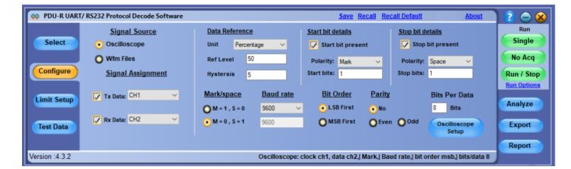
For easy and quick analysis, PDU-R offers flexibility to display the order of MSB and LSB bit in decoded byte. User can define number bits per data byte makes PDU-R a customizable view of the decoded data. These features make PDU-R software industry best decode and debug UART signals.
