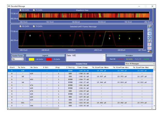
PDU-R with DPO70000/DSA70000 high bandwidth oscilloscope series can be used to debug the UART/RS232 serial buses. This enables designers to use DPO/DSA70000 series oscilloscopes for debugging of UART/RS232C signals along with high speed designs SATA/DDR/HDMI/FBDIMM/PCI-E and so forth.
