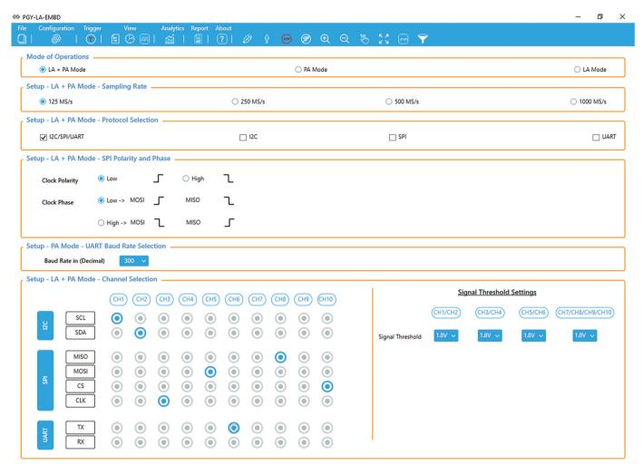
Users can easily configure the Logic Analyzer for embedded interfaces by either selecting Logic Analysis (LA) mode or Protocol Analysis (PA) mode or a combined (LA+PA) mode. This ensures a quick and easy way to configure the product and look at complex problems at system level either in Logic Analysis (State Analysis, Timing Analysis) or Protocol decoding or both. Save and Recall capability ensures designers can recall their custom setup details.
