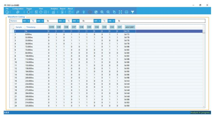
State view helps designers to see the actual signal behavior. Using the device clock as reference, it provides the plot of clock and data signals with bus diagram. Grouping of signals ensures designers have the flexibility to view signals together. All signals are time correlated to help look into setup and hold times, pulse width, missing data etc. which are very critical for digital designs as designers look to optimize their codes.
