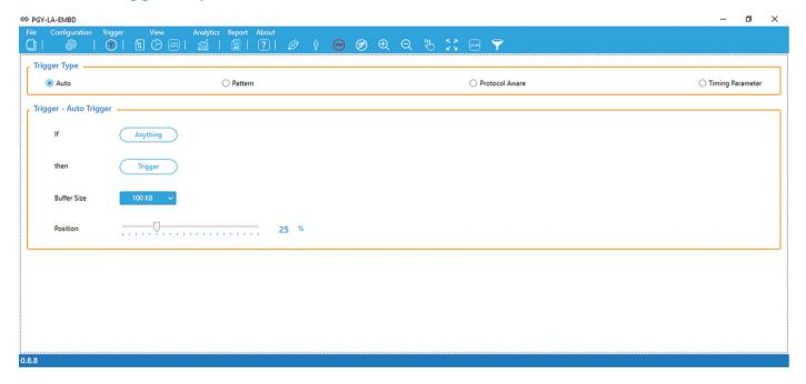
PGY-LA-EMBD supports Auto, pattern, Protocol aware and timing parameter trigger capabilities. Users can trigger on any of the Protocol packets. Comprehensive Trigger provides the flexibility to monitor different conditions.
