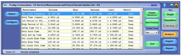
PGY-I2C runs inside the Tektronix oscilloscopes and makes the electrical measurements, decodes protocols and displays the decoded data in a bus diagram, a table, and links the decoded data to electrical signal in the bus diagram. I2C Protocol-based trigger can be se tup using the built-in I2C trigger capabilities in Tektronix oscilloscopes.
