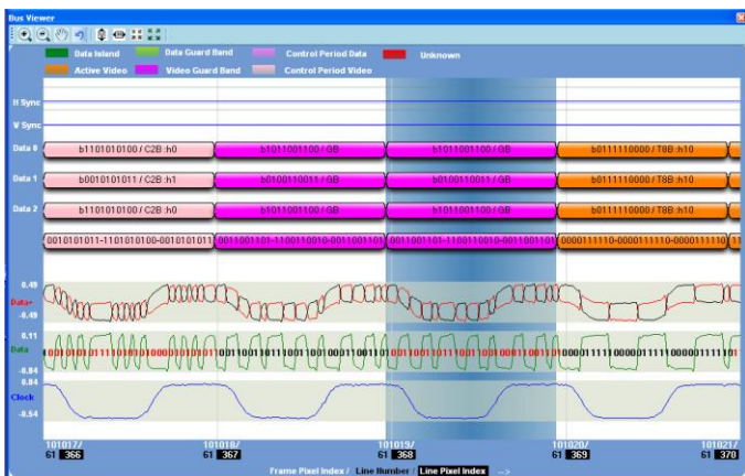
Figure 5: MHL Bus viewer with Physical layer waveforms
